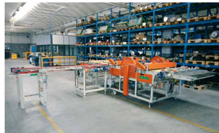
Raccoglitore pressa, rulliera di carico essiccatoio, e trasporto trasversale di by-pass. Press reception unit, drier loading roller way and transverse by-pass conveyor. Colector prensa, rodillera de carga secadero y transporte transversal de by-pass. Ramasseurs presse, chemin à rouleaux de chargement séchoir et transport transversal de by-pass.
