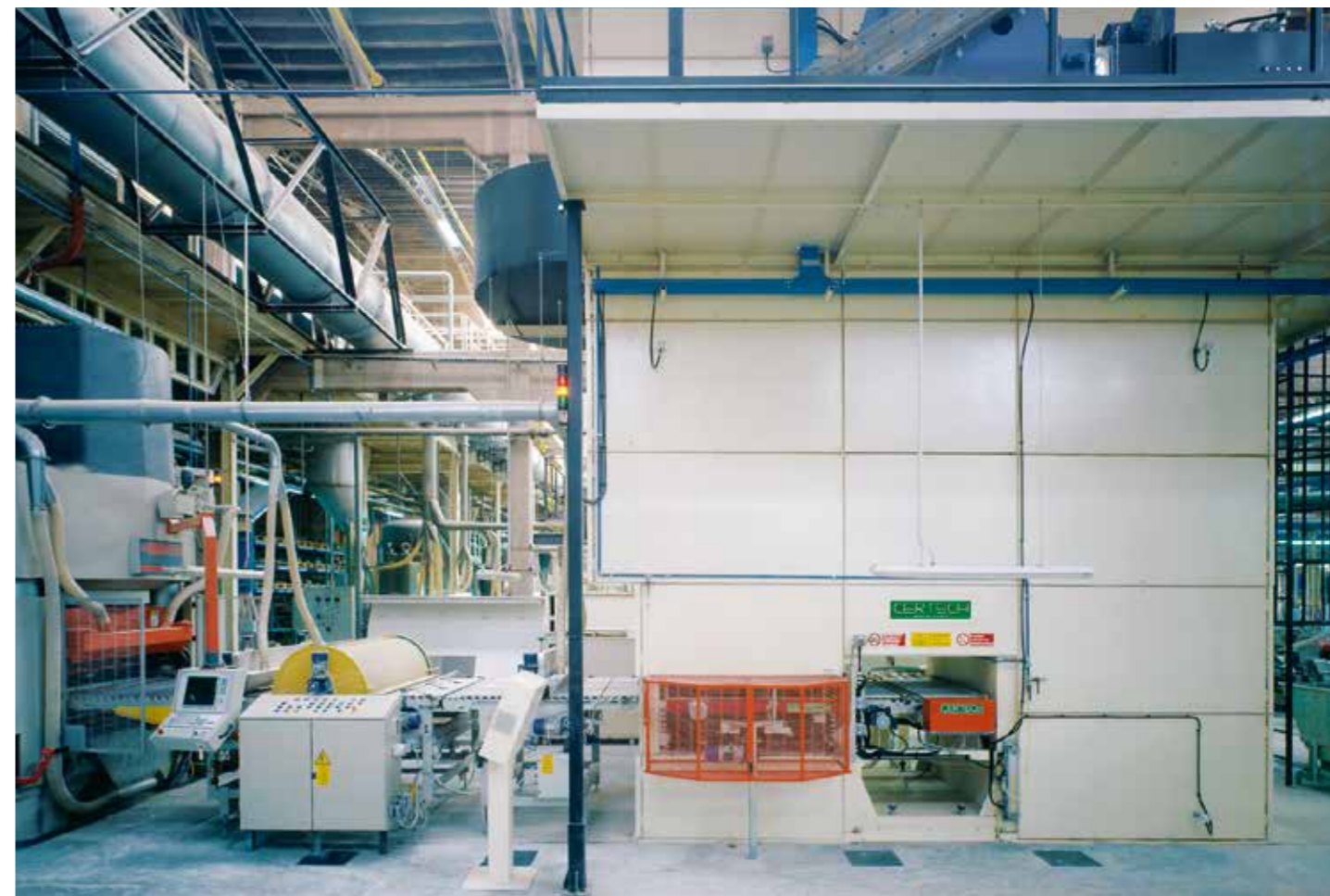
Essiccatoio verticale RVD 16M-1350. RVD 16M-1350 vertical drier. Secadero vertical RVD 16M-1350. Séchoir vertical RVD 16M-1350.
